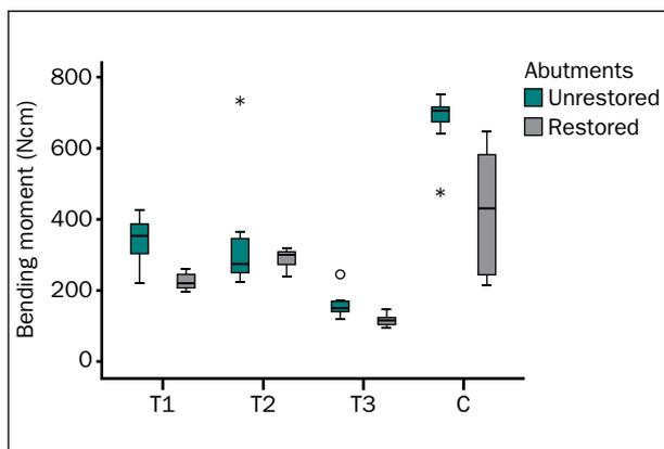
**Fig 2** Bending moments of tested unrestored and restored abutments after static loading.
