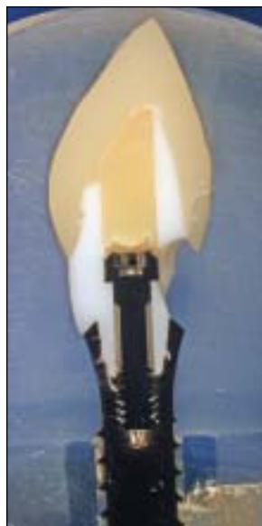
**Fig 7c** Abutment fracture above the implant shoulder in T3.
