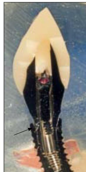
**Fig 7d** Plastic deformation of a control implant-abutment complex with fracture of the implant (arrow).
