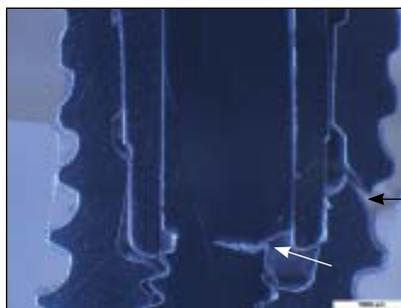
**Fig 5** (Left) Fracture mode in T3. The fracture line on the abutment is above the implant shoulder.
